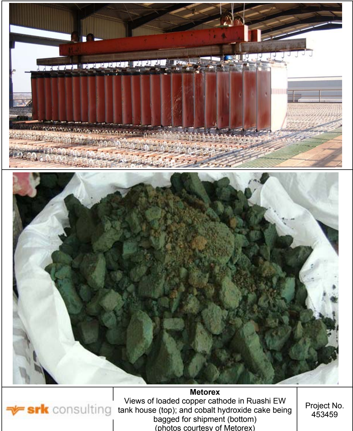
Figure 3.27: Views of loaded copper cathode in Ruashi EW tank house (top); and cobalt hydroxide cake being bagged for shipment (bottom)
