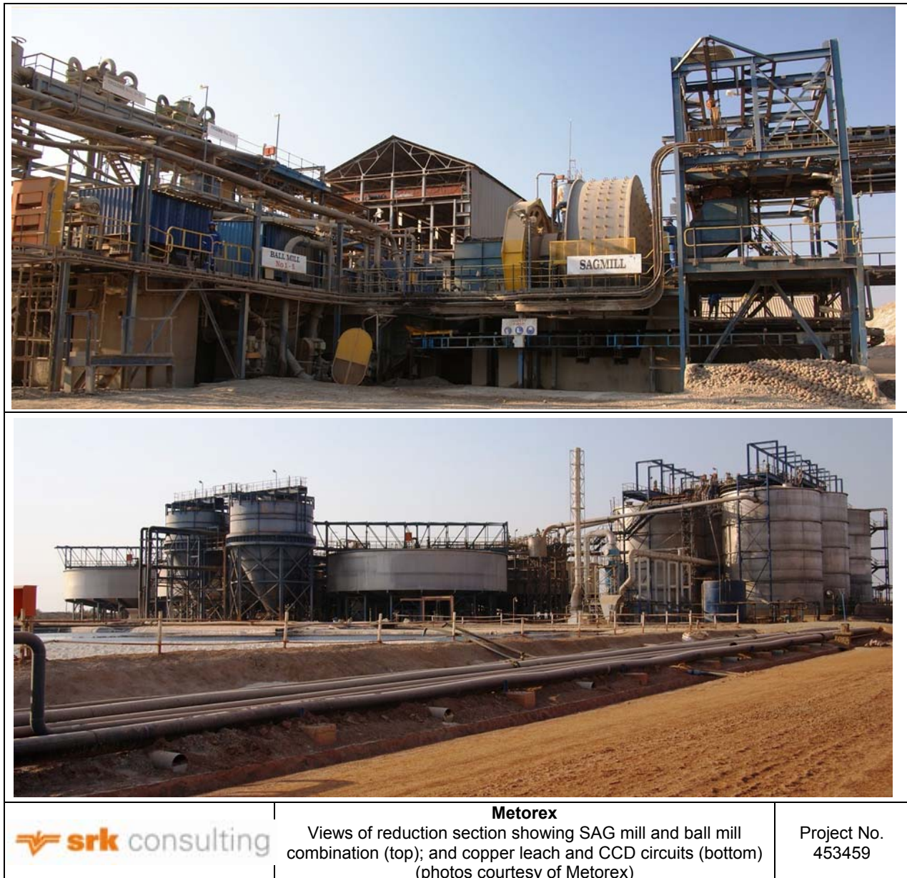
Figure 3.26: Views of reduction section showing SAG mill and ball mill combination (top); and copper leach and CCD circuits (bottom)
