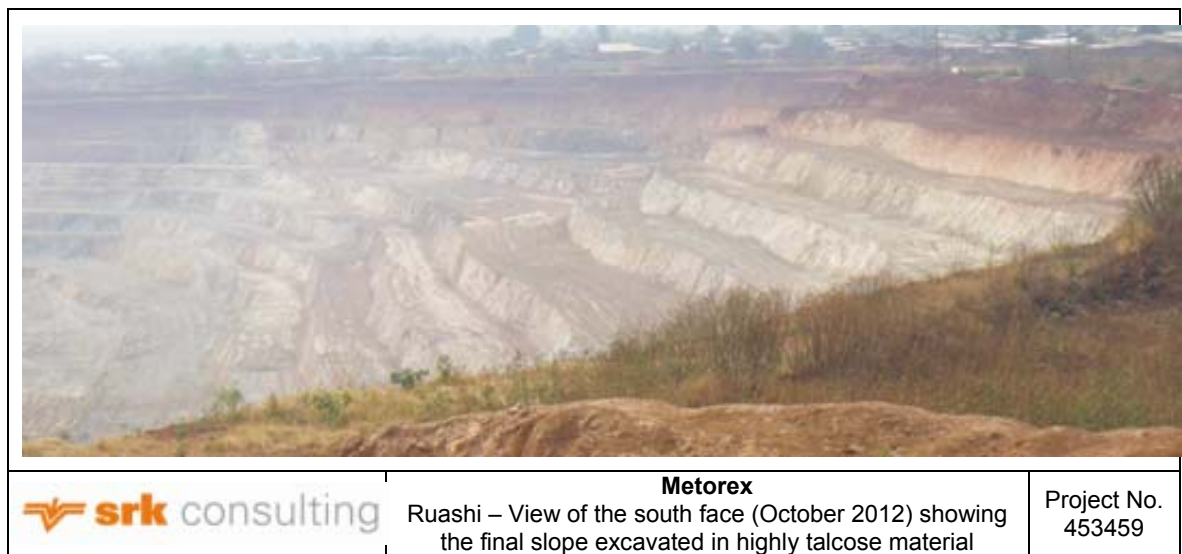
Figure 3.20 Ruashi – View of the south face (October 2012) showing the final slope excavated in highly talcose material
